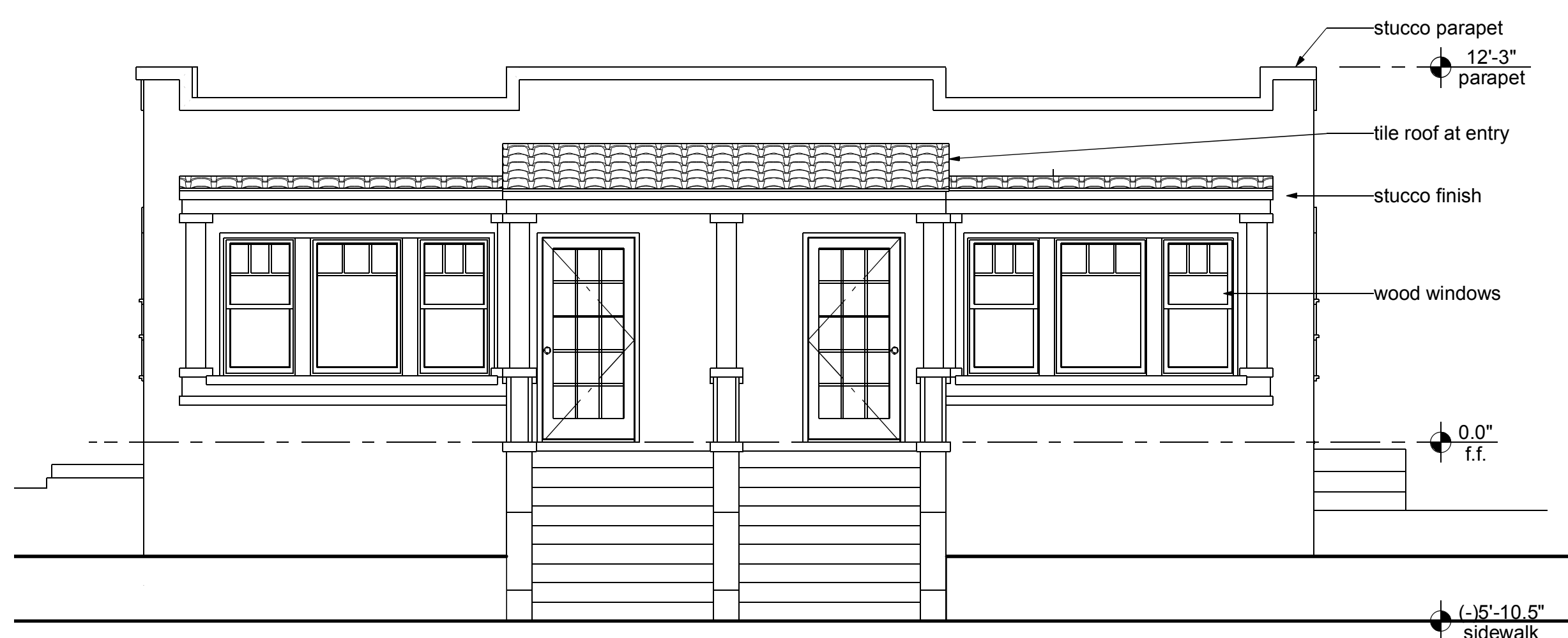
2 Existing West Elevation - Front
